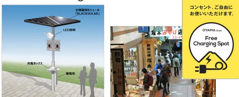
The diagram shows a solar charging station (ソーラー充電スタンド) with a solar panel (太陽電池モジュール「BLACKSOLAR」), LED lighting (LED照明), a charging socket (充電ボックス), and a battery (蓄電池). An arrow points to a QR code sticker with the text 'OYAMA Area Free Charging Spot' and 'コンセント、ご自由にお使いいただけます。' (You can use the socket freely).
